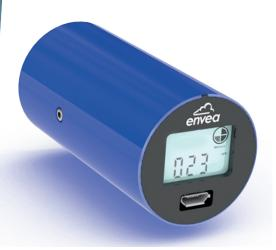
Most of the Cairsens® sensors use amperometric technology consisting of three electrodes: the working electrode (anode), the counter electrode (cathode) and the reference electrode. The gas to be analyzed is diffused through a permeable membrane towards the sensitive electrode. The function of the gas, oxidation takes place at the anode, or reduction at the cathode. The electrical signal generated between the two electrodes is proportional to the concentration.
